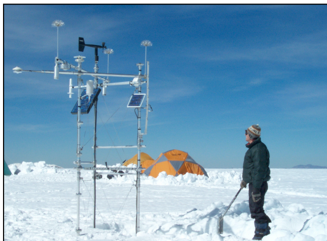
Prof. Vuille working on an automated weather station at 5760 m in the Peruvian Andes
