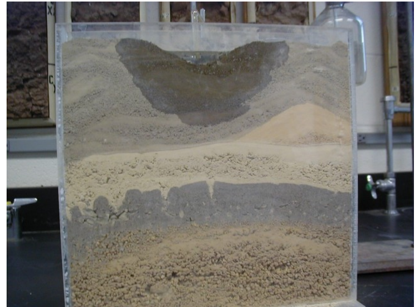
Saturation from above. Note percolation to lower layers.
