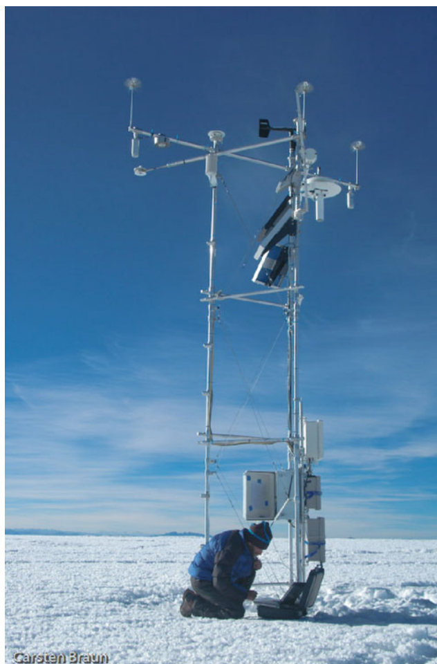
Climate Variability and High Altitude Temperature and Precipitation, Figure 1 Automated weather station (AWS) on the summit of Quelccaya ice cap, located at 14°S in the eastern Peruvian Andes (Cordillera Vilcanota) at 5,670 m above sea level. Photo courtesy of Douglas R. Hardy.
