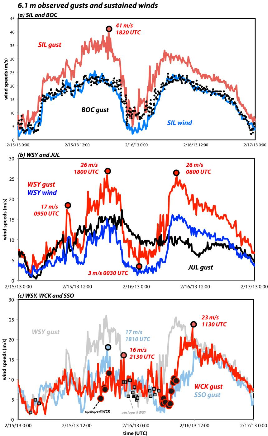
FIG. 6. Time series of observed gusts and sustained winds ( $\text{m s}^{-1}$ ) over 2 days at (a) SIL and BOC; (b) WSY and JUL; and (c) WSY, WCK, and SSO. Some maxima and minima are highlighted. In (c), black dots indicate times when winds were directed upslope at WCK and gray squares indicate times when winds were directed upslope at WSY.
