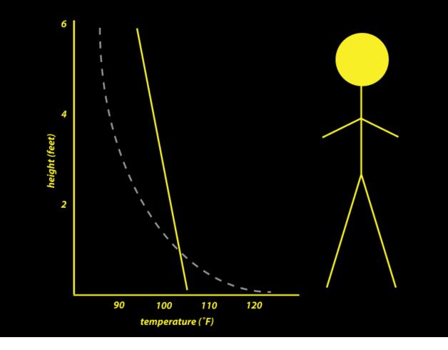
At night, the sand's low thermal inertia permits it to get cold. This chills the air near the ground but warmth from aloft is not conducted quickly downward, again owing to air's poor conductivity.
