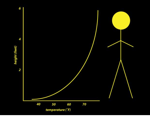
This figure reveals a **temperature inversion**... the opposite (inverse) of what we expect. It's also called a **radiation inversion**, caused by radiative cooling of the sandy surface, exacerbated by sand's low thermal inertia and air's poor heat conductivity.
