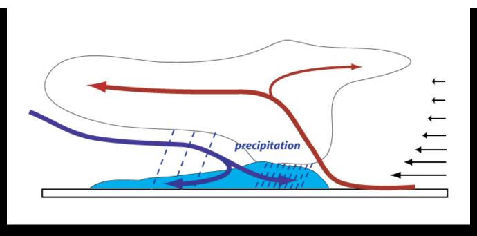
Note the rear inflow descends to the surface as it moves forward. This is because of precipitation. Specifically, precipitation that EVAPORATES and makes the rear inflow air COLD and NEGATIVELY BUOYANT. Sometimes the descending rear inflow can bring extremely strong winds to the surface and cause a lot of damage.
