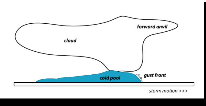
We see the FORWARD ANVIL at upper right. Below the cloud shield is the SUBCLOUD COLD POOL. It's very much like a cold front, but usually much stronger. The leading edge of the cold pool is called the "gust front". The wind gusts pick up after it passes you.
