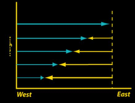
• We have changed the frame of reference to that of the squall line, which is propagating eastward faster than the westerly winds in which it is embedded.
