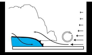
But the storm isn't leaning downshear. Why not? Note the circulation around the cold pool. This negative buoyancy also produces a circulation, and it's directed CCW from our point of view, OPPOSITE to the shear's induced circulation.
