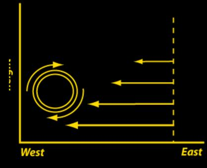
But the point is we STILL have westerly vertical wind shear, and the shear STILL wants things to spin CW in this vertical plane
