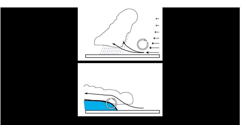
With only the cold pool, and no shear, the inflowing air might be lifted to saturation, but it will also be accelerated quickly rearward by the pool circulation, severely LIMITING its lift.
