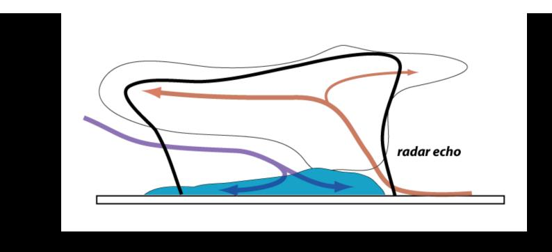
This is the part of the storm visible to 10 cm weather radar -depending on how far from the radar it is, of course.
