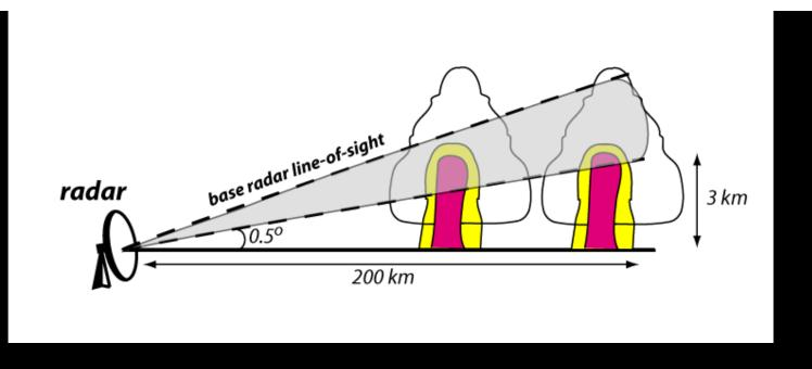
Weather radars are at the ground and look up as well as out, starting at a small angle to the horizontal.
