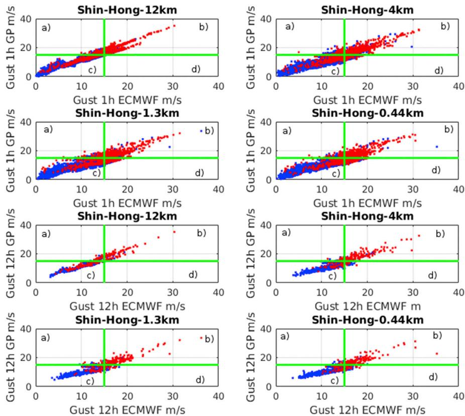
Fig. 18. ECMWF vs. GP (m/s) gust forecasts at the RM tower, using the Shin-Hong PBL scheme at 12 km, 4 km, 1.33 km, and 0.444 km horizontal grid resolution, and time windows of 1-h (top) and 12-h (bottom). Red dots show gusts exceeding  $g > 15$  m/s over the time interval being considered. (For interpretation of the references to color in this figure legend, the reader is referred to the Web version of this article.)
