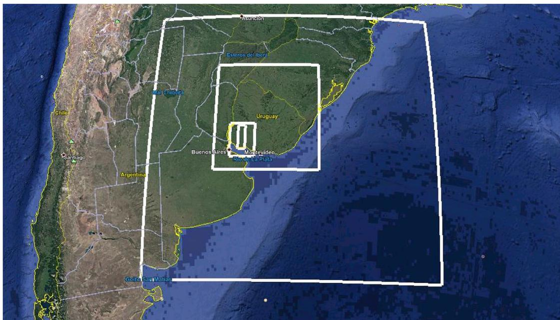
Fig. 10. Telescoping Weather Research and Forecasting (WRF) domains with horizontal grids of 12, 4, 1.33, and 0.444 km.
