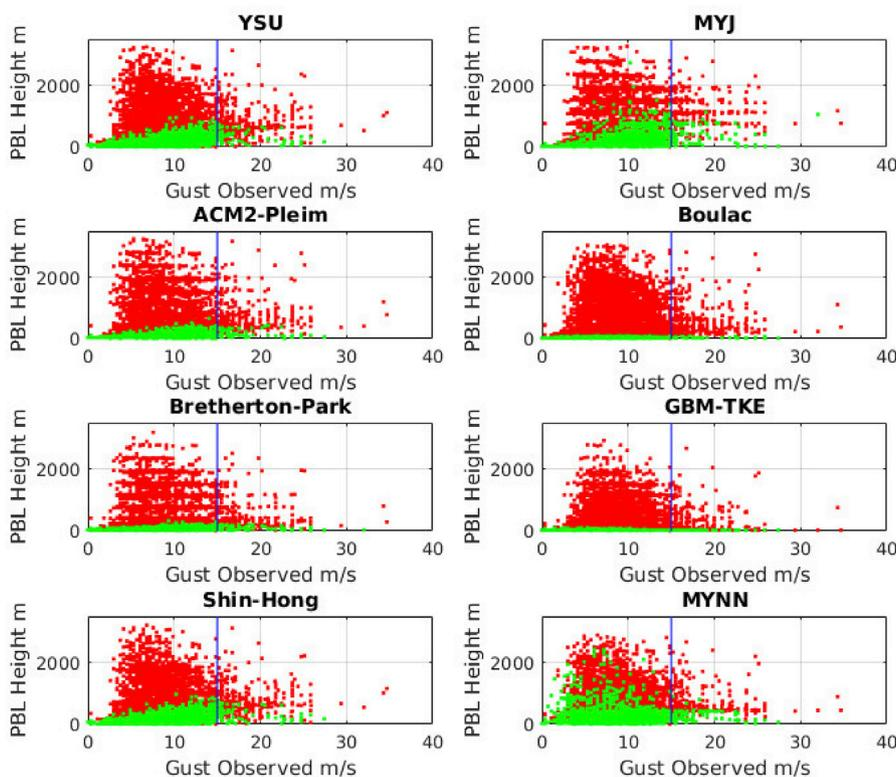
Fig. 14. Predicted PBL heights vs. observed gusts for the CE tower location, from 4-km WRF simulations using the eight PBL schemes. Green dots indicate strongly stable conditions ( $\frac{\partial T}{\partial z} > 0$ ), computed from the simulations. Large gust (15 m/s) threshold indicated. (For interpretation of the references to color in this figure legend, the reader is referred to the Web version of this article.)
