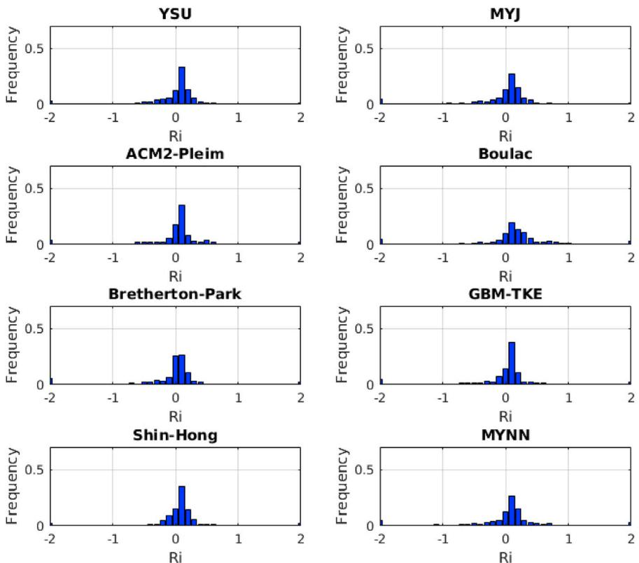
Fig. 13.  $Ri$  computed from 4-km WRF simulations using the eight planetary boundary layer schemes at CE tower when the observed gust was  $> 15$  m/s.
