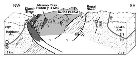
Figure 4. Northwest-southeast cross section through Nanga Parbat; section line extends along Diamir gah, through summit and south of lower Rupal valley. Lithologic patterns are in Figure 1. MMT is Main Mantle thrust.
