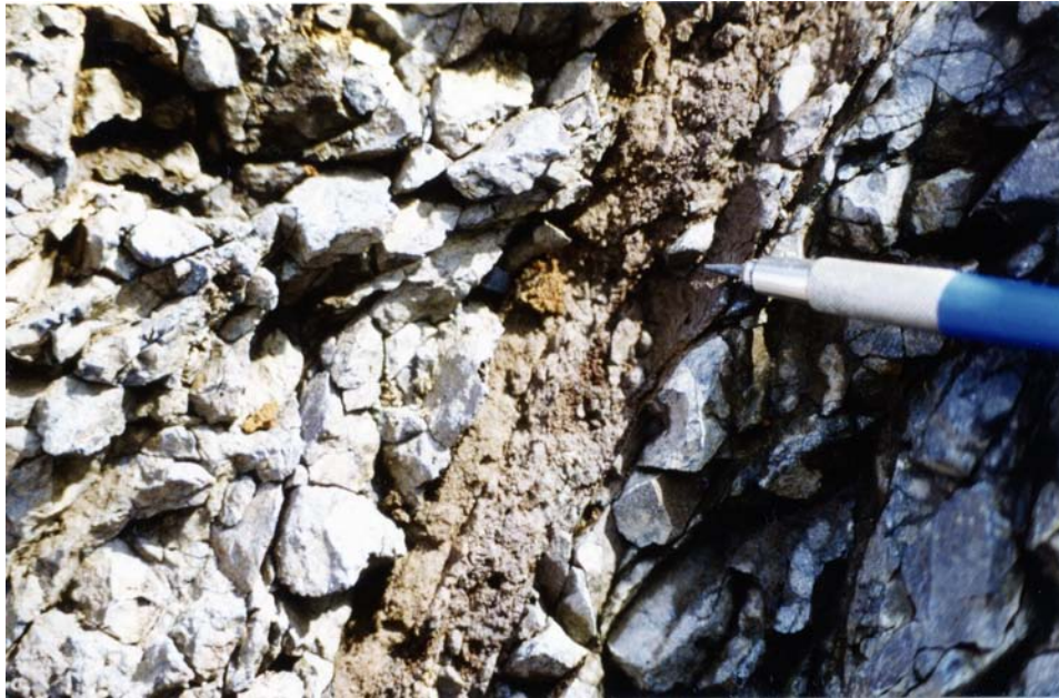
Figure 3.34. Close up of fault zone shown in Figure 3.31, showing oblique fault gouge foliation which is here interpreted as a result of dextral motion along the Northern Arm Fault.
