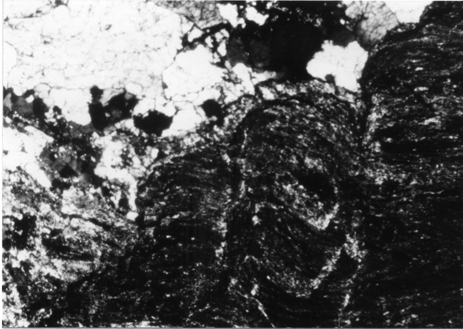
Figure 5.19. - Thin section photograph of crenulation cleavage deforming a quartz vein.
