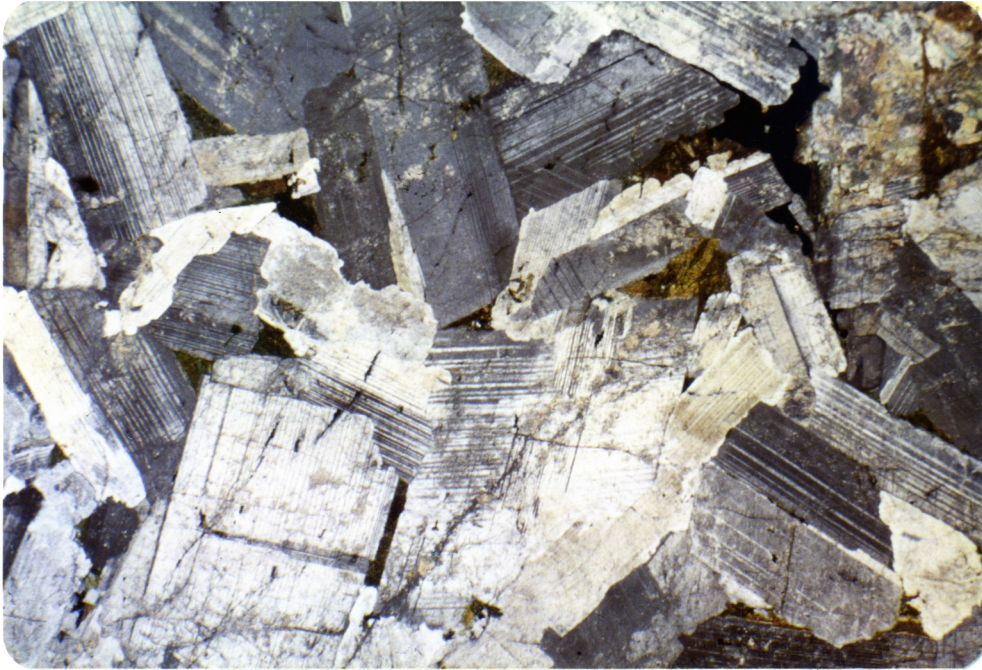
Figure 7LL - Photomicrograph of typical isotropic gabbro showing randomly oriented plagioclase laths.
