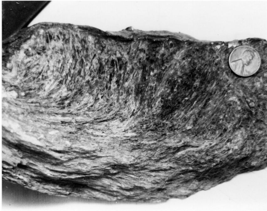
Figure 34 – Typical podiform body of actinolite from the “blackwall” zone. The upper surface of the specimen is the contact with the biotite-chlorite schists, while the lower surface faces inward toward the talc zone. Actinolite needles are deformed into the foliated talc in the center of the specimen.
