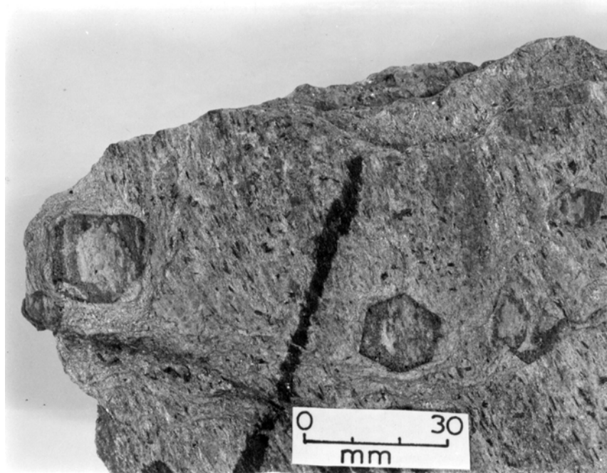
Figure 12 – View of tabular garnets normal to S_2 layering. The garnets, though sliced into tabular sections within the foliation, are equidimensional in this plane. The nearly vertical L_2 lineation indicates the trace of S_1 layering in which the garnet growth occurred. The absence of quartz striping parallel to the lineation on the surface of the garnets indicates no slicing occurred in S_1 in this example.
