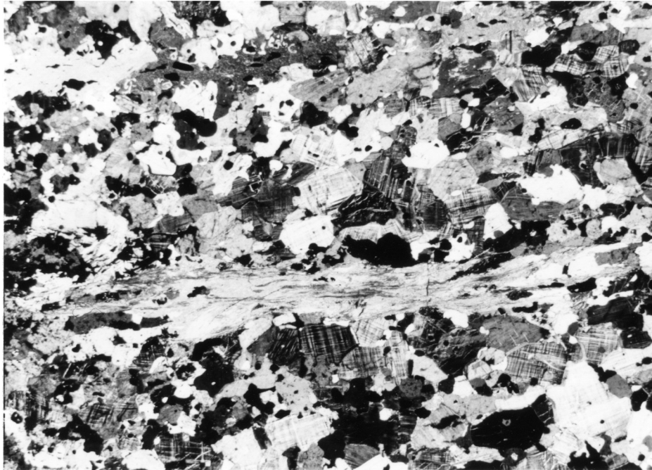
Figure I-4. Photomicrograph of Noduliferous Microcline Granitic Gneiss. Elongate mass in center is small quartz-sillimanite nodule. Long dimension of photo is 1.75 cm..
