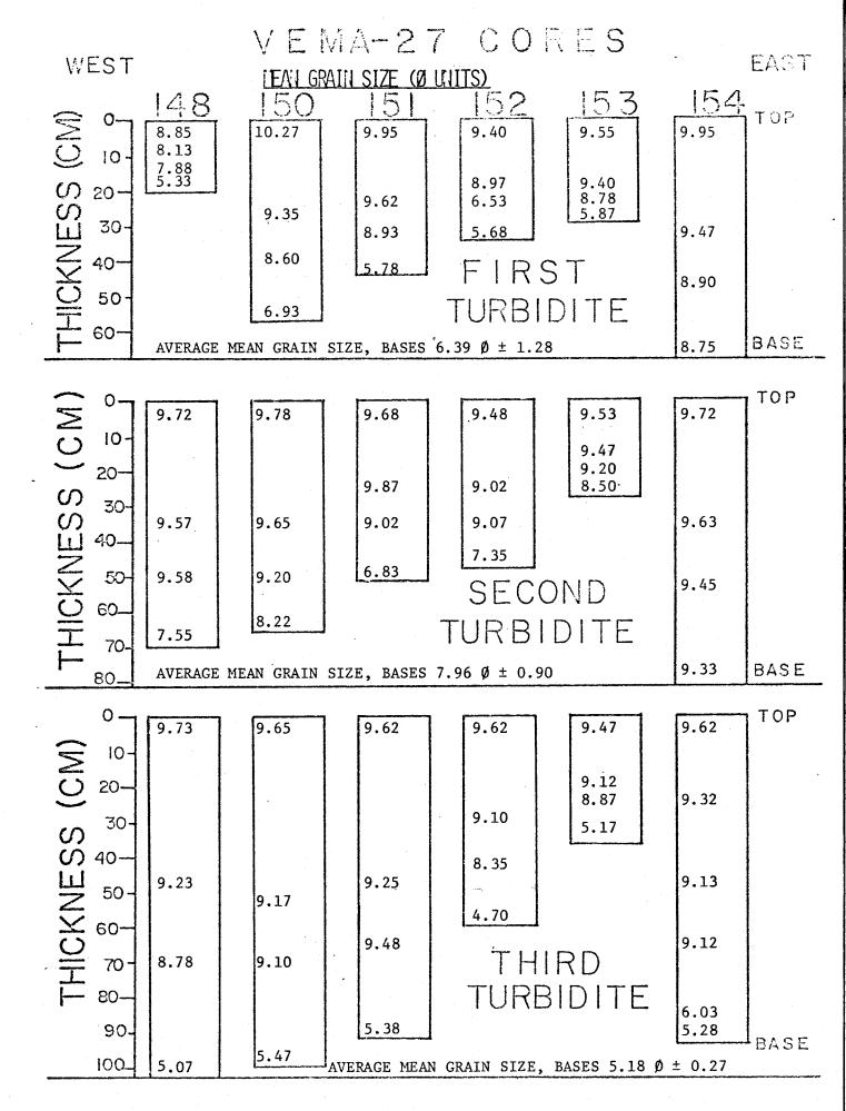
displays this general trend; the third turbidite follows this same trend, except that cores 150 and 148 are slightly thicker than 154. Based on the average thicknesses of each of these turbidites and the areas they cover (15000  $\rm km^2$ ), the calculated turbidite volumes are: first turbidite, 5.7  $\rm km^3$ , second turbidite, 8.0  $\rm km^3$ , and third turbidite, 12.1  $\rm km^3$ .
