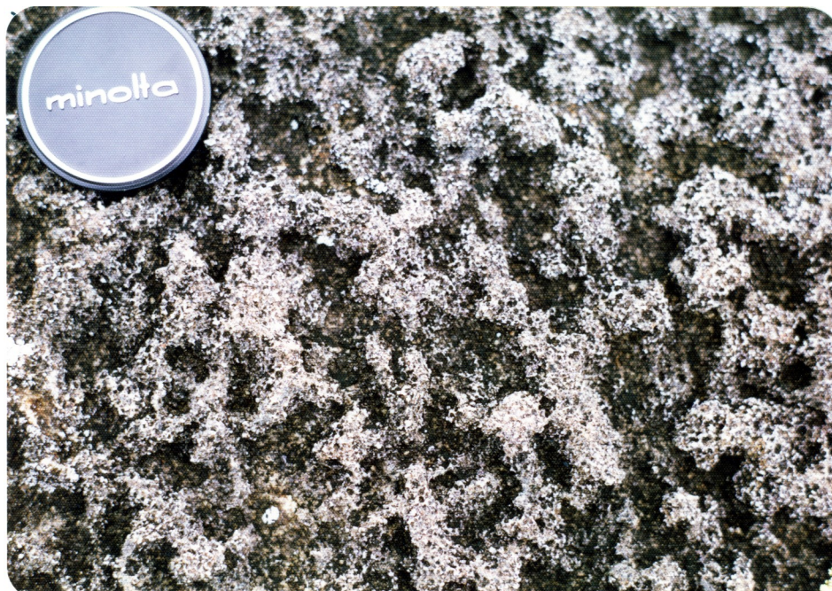
Figure 32 Spongy surface texture of the feldspathic lherzolite with plagioclase (white) oikocrysts enclosing small, less resistant olivine grains (gold); dark green material is clinopyroxene, orthopyroxene or amphibole (pargasite?) oikocrysts.
