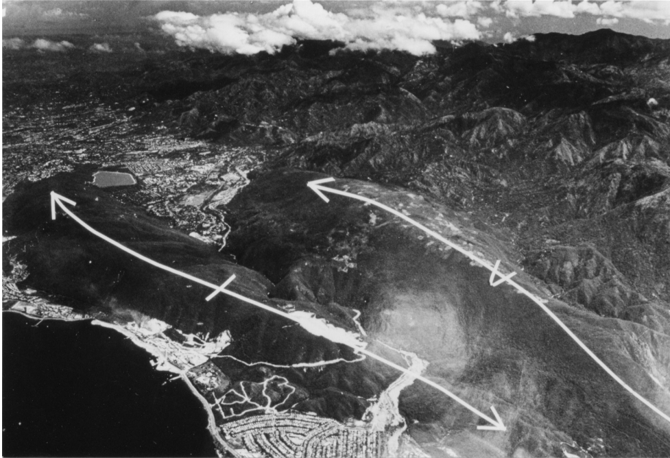
Figure 6. Aerial view of southwestern margin of the Wagwater Belt adjacent to Kingston. Wagwater Fault Zone is a steep reverse fault (see Section D, Figure 5) along which the Paleogene sedimentary (Wagwater and Richmond Formations) and volcanic rocks (Newcastle Volcanics) of the Wagwater Belt overthrust the alluvial plain on which the city of Kingston is built. Overthrusting has produced folding in rocks as young as Pliocene (fold axes indicated). Note the difference in topography produced by the Wagwater Belt lithologies (i.e. the Newcastle Volcanics being the most resistant to erosion and the Richmond Formation being the least resistant).
