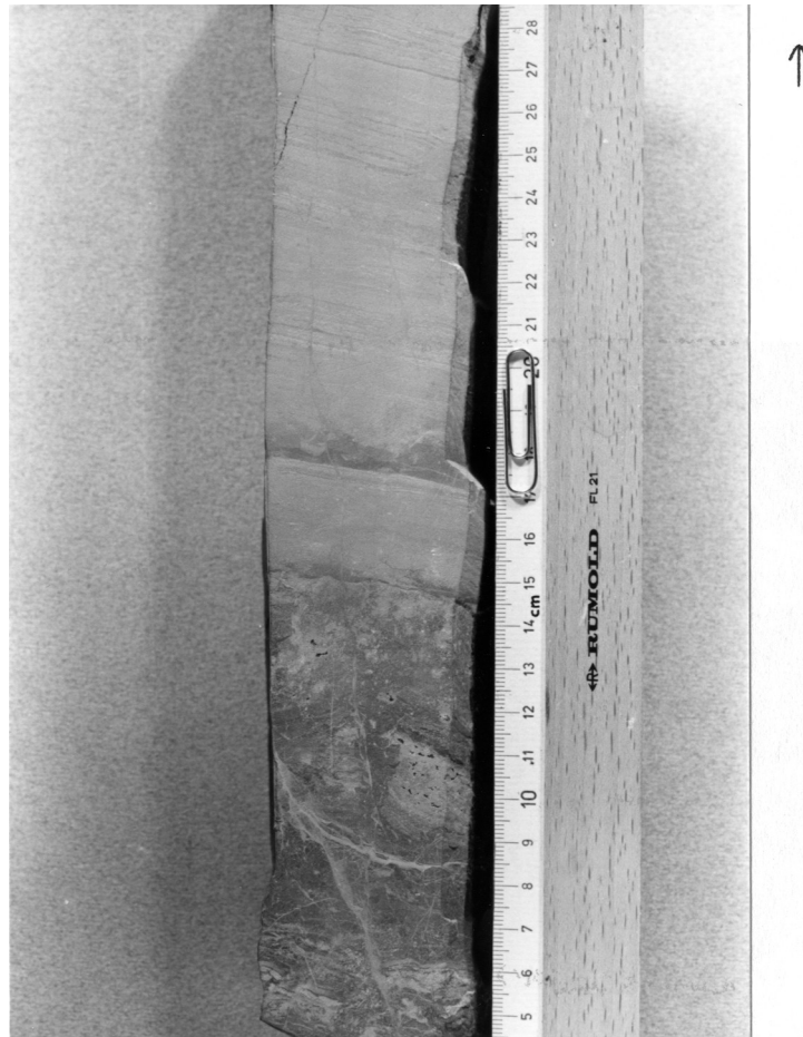
Fig. 2.5.- Polished and etched slab of dolostone showing a "shallowing-up" sequence. Note mottled (below; lower intertidal) and mudcracked laminated (above; upper intertidal) facies. Mudcracks appear as laminae discontinuities. Isle La Motte Section (18.5 m). Arrow indicates top.
