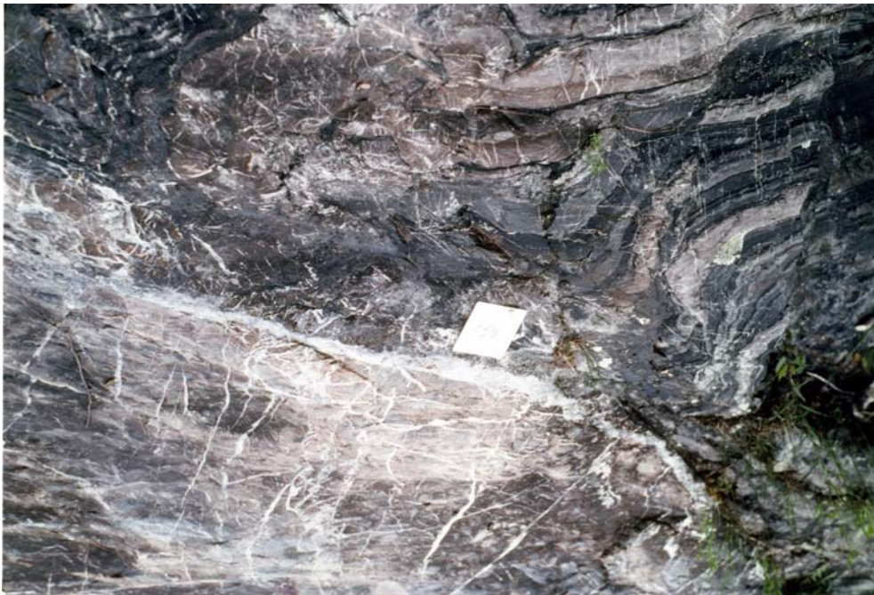
Figure 4.16. Same outcrop as 4.15 showing region where fault cross-cuts bedding and is associated with folding and disruption of bedding as well as extensive veining shown in Figure 4.17. White plaque is 10 cm on an edge.
