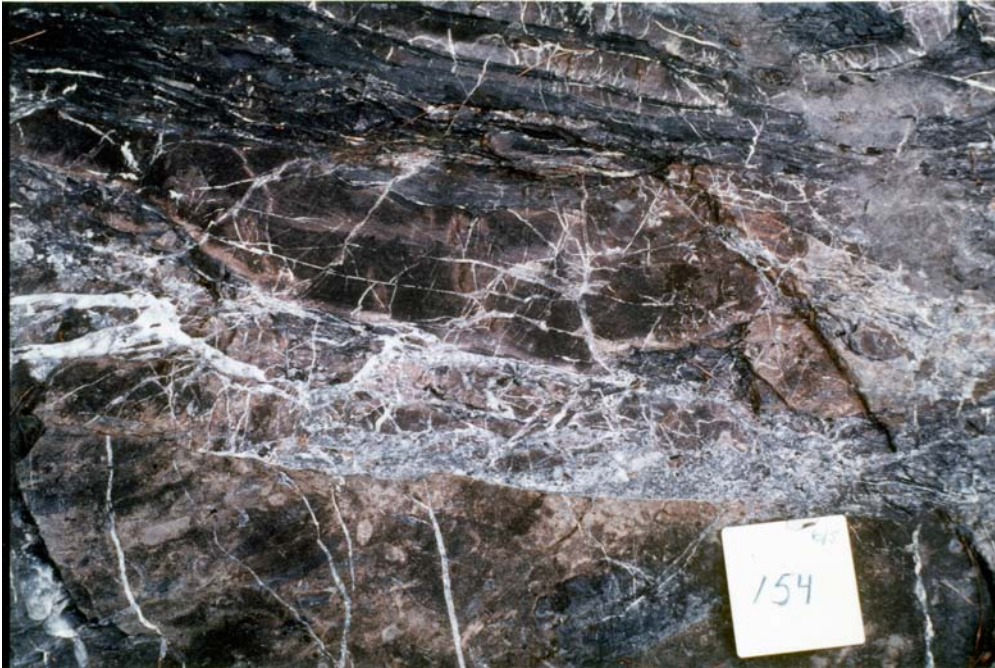
Figure 4.17. Close-up of a region where the fault surface obliquely intersects thicker dolomitic quartz arenite layer. Note the development of net veining in the arenite.
