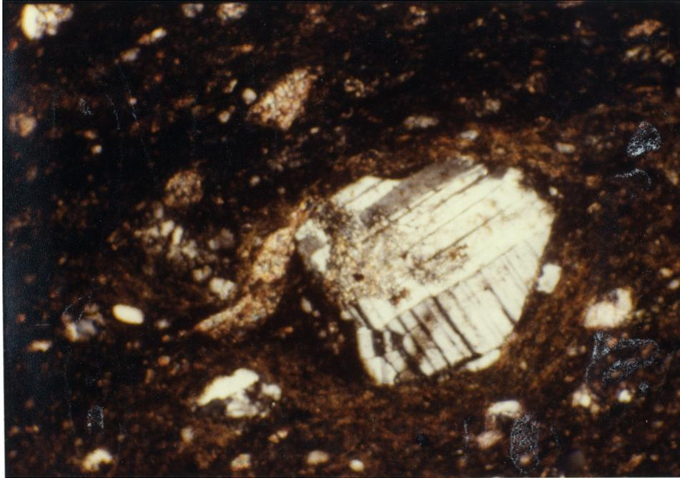
Fig. III-3: Complex plagioclase twinning in the metamorphic tuff.
