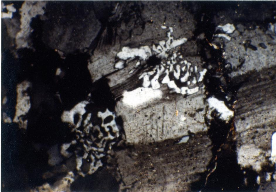
Fig. III-1: Myrmekitic texture in high-K granite (alaskite). Albite exsolution forms the myrmekitic texture in the perthite.
