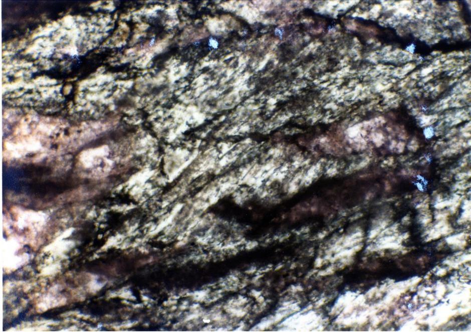
Fig. IV-5-E: Shear-band foliation in the Lower Supra-Err Slice.
