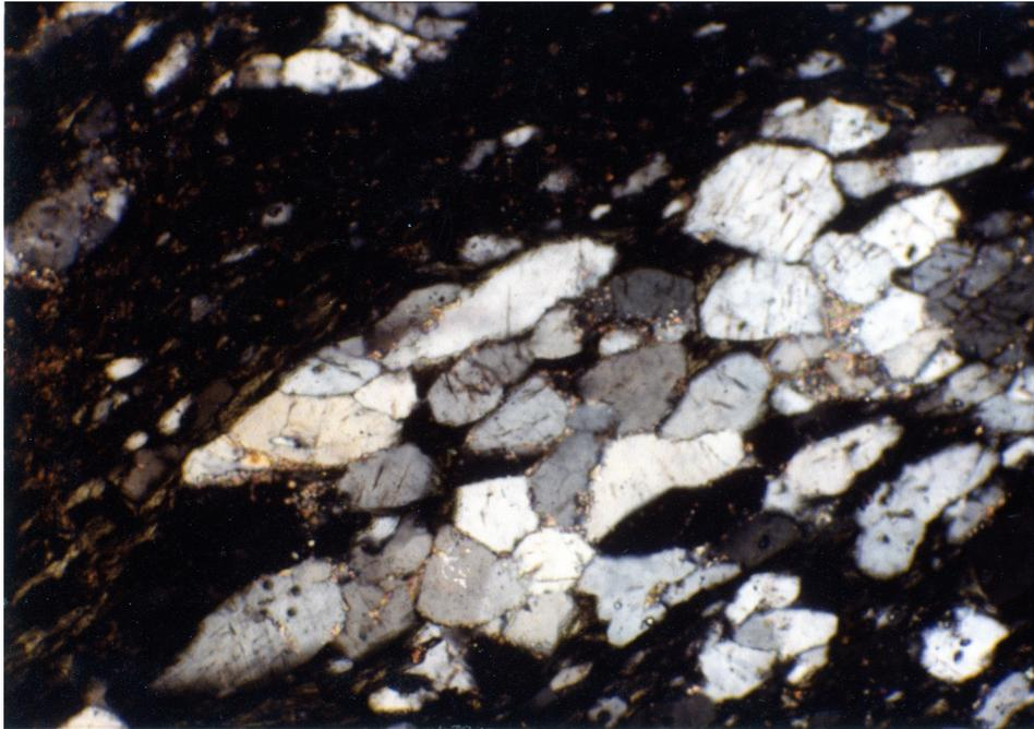
Fig. III-7: Quartzite with partially recrystallized quartz vein.
