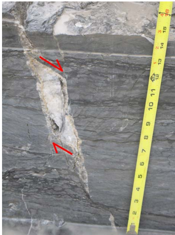
Figure 34 - Rhombohedral pull-apart with red arrow to indicate motion direction (taken from eastern wall of trench 6)
