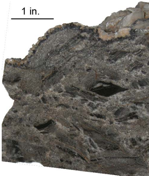
Figure 26 – Cross-section of a brecciated block from inside dolomite body
