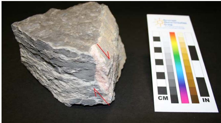
Figure 35 - Calcite/dolomite rhomb with slicken-sides taken from the quarry
