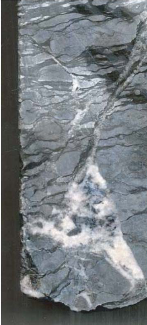
Figure 41 - Calcite mineralization in a fracture from Hole 2 core at 31 ft.
