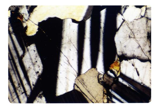
Figure 2. Sample 308A, crossed nicols. Photomicrograph showing the general adcumulus nature of plagioclase crystals with interlocking boundaries. The small intercumulus grains of olivine are typical of many adcumulus-mesocumulus textured samples in this study. Olivine is a major primary phase elsewhere in this slide, suggestive of co-precipitation of olivine and plagioclase.
