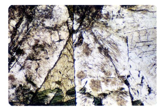
Figure 3. Sample 123B, plane light. Photomicrograph showing orthocumulus texture with amphibole (note cleavage) interstitial to interlocking subhedral-euhedral plagioclase laths. Note that the more sodic rims of the zoned plagioclase are less altered than the more calcic cores.
