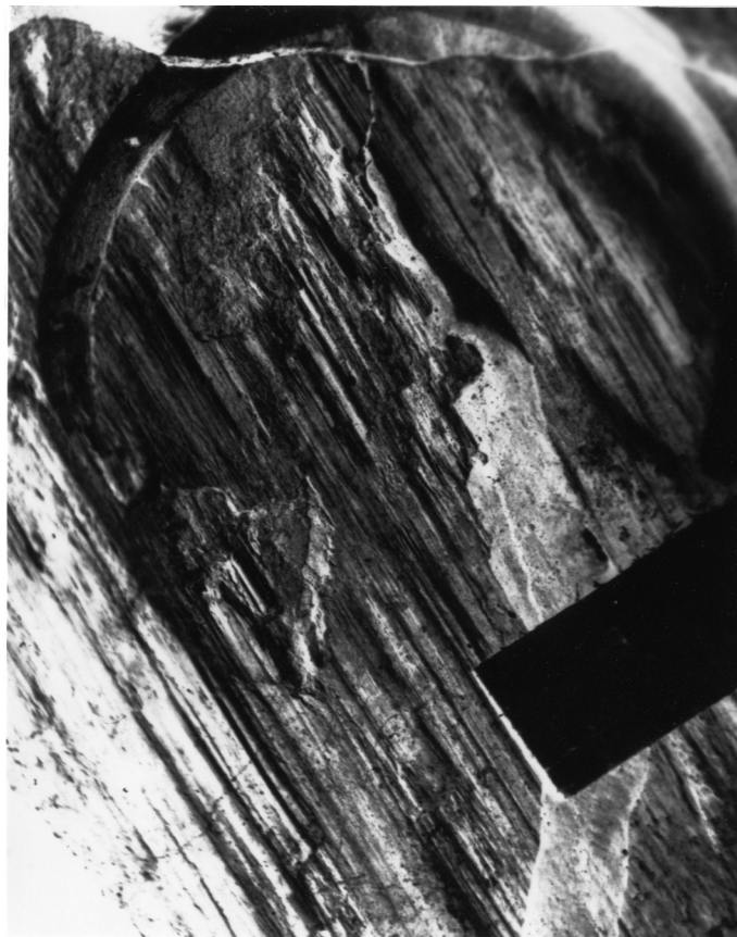
Figure 42. Demonstration of nesting using the reversed print technique. Same specimen as in figure 40. The specimen broke apart before the technique was applied and was glued together with epoxy. The epoxy causes the fuzzy appearance in the center of the reversed print.
