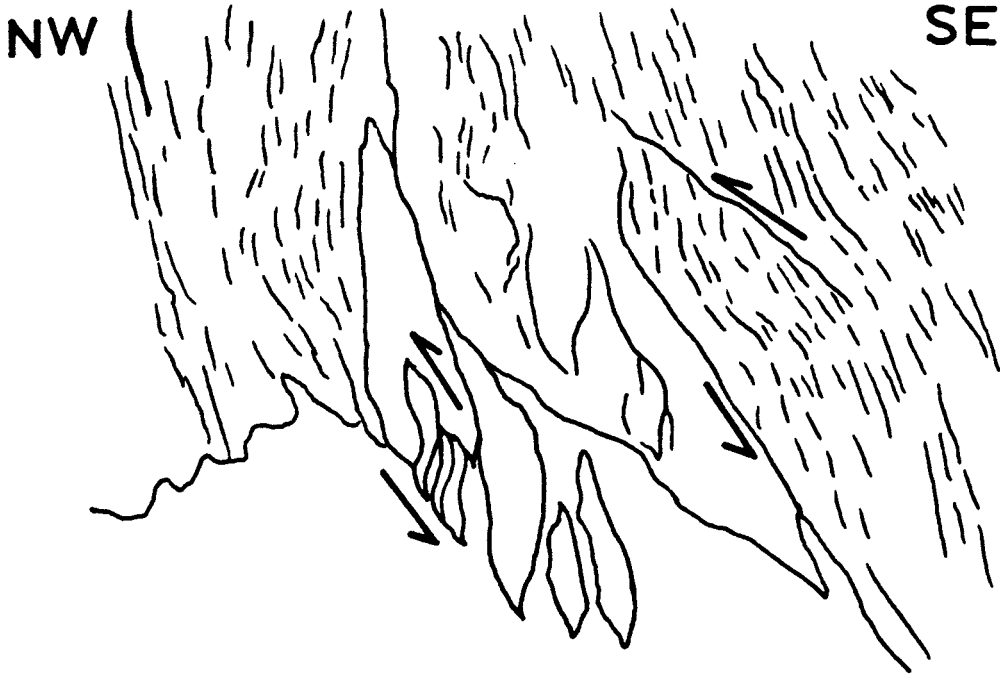
Figure 5.7 Bending phenomena of rock chips between small faults associated with the basal thrust of the Taconic Allochthon.
