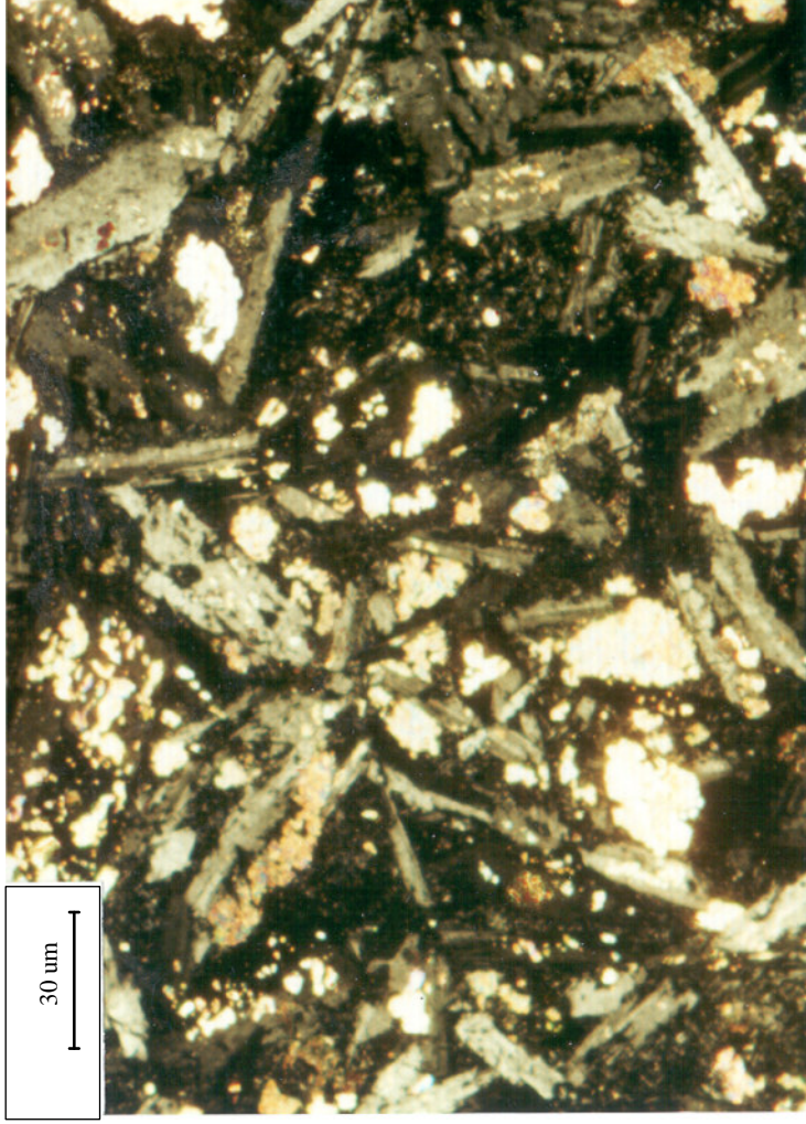
Figure 3. 18 Photomicrograph of a volcanic rock fragment composed of plagioclase phenocrysts within fine-grained ground mass. This indicates that there was a significant volcanic source for the Tianba Flysch.
