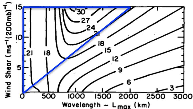
FIG. 7. Maximum growth rate ( $10^{-6} \text{ s}^{-1}$ ) plotted as a function of wind shear in the 700–900 mb layer and wavelength for the BCD/CISK mode with  $f_8 = 0.7$ .
