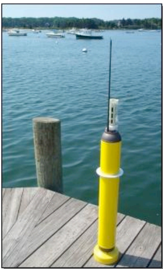
Drifting profiler shown before deployment. Instruments of this type make Lagrangian measurements as they are swept along by ocean currents. Satellites track their positions with Global Positioning Systems (GPS).
