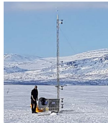
Fieldwork on a frozen lake. Micrometeorological mast installed on Lake Torneträsk.
