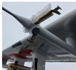
Ice accumulated on the Nevzorov probe on the wing of the Convair-580 following IOP9 flight 1.
