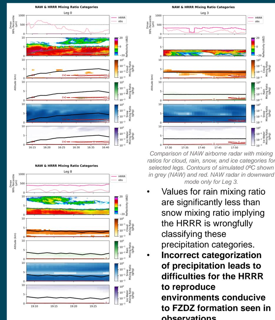
Comparison of NAW airborne radar with mixing ratios for cloud, rain, snow, and ice categories for selected legs. Contours of simulated  $0^{\circ}\text{C}$  shown in grey (NAW) and red. NAW radar in downward mode only for Leg 3.
